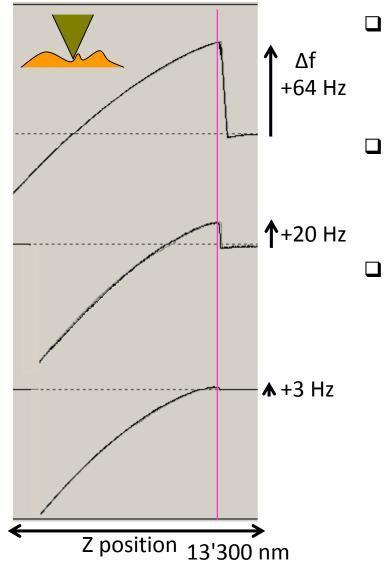
In the quasi contact mode, the tip is always in contact, but the TF is still vibrating. Hence, one can measure an extremely large displacement, which is several hundreds of micro or more.
